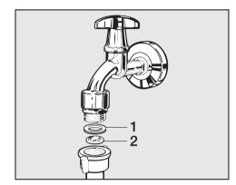
plastic filter, **2**, and pull it out of the hose connector.
